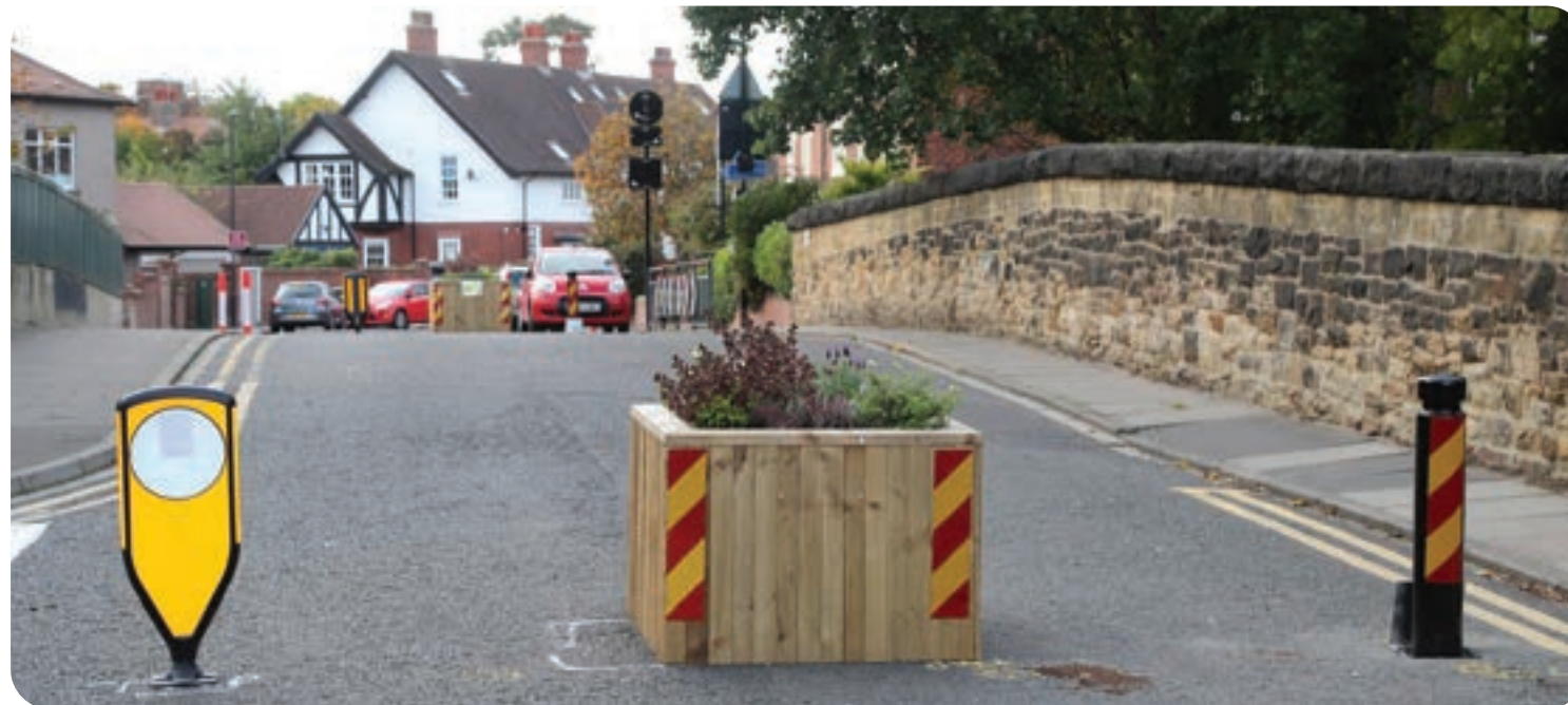
Planters such as the one used on Stoneyhurst Bridge could be installed to restrict traffic in neighbourhoods.
